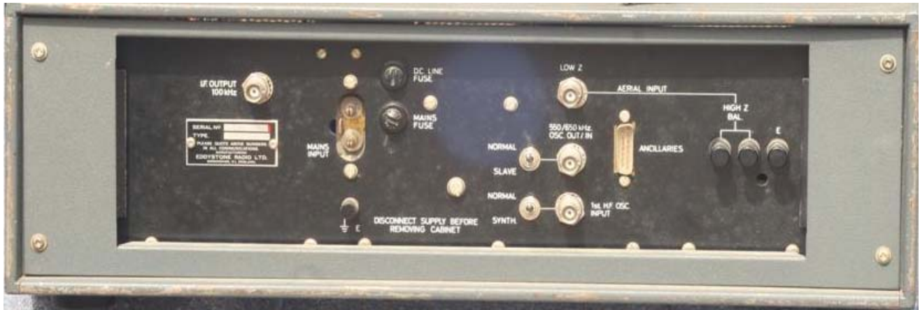
Above: close-up of the EC958 rear panel – 'wot, no chocolate block...' Below: Internal view of a EC958 – note absence of the 10KHz calibrator module present in the EC958/3, where it sits atop the incremental oscillator unit (see photo on page 26)
