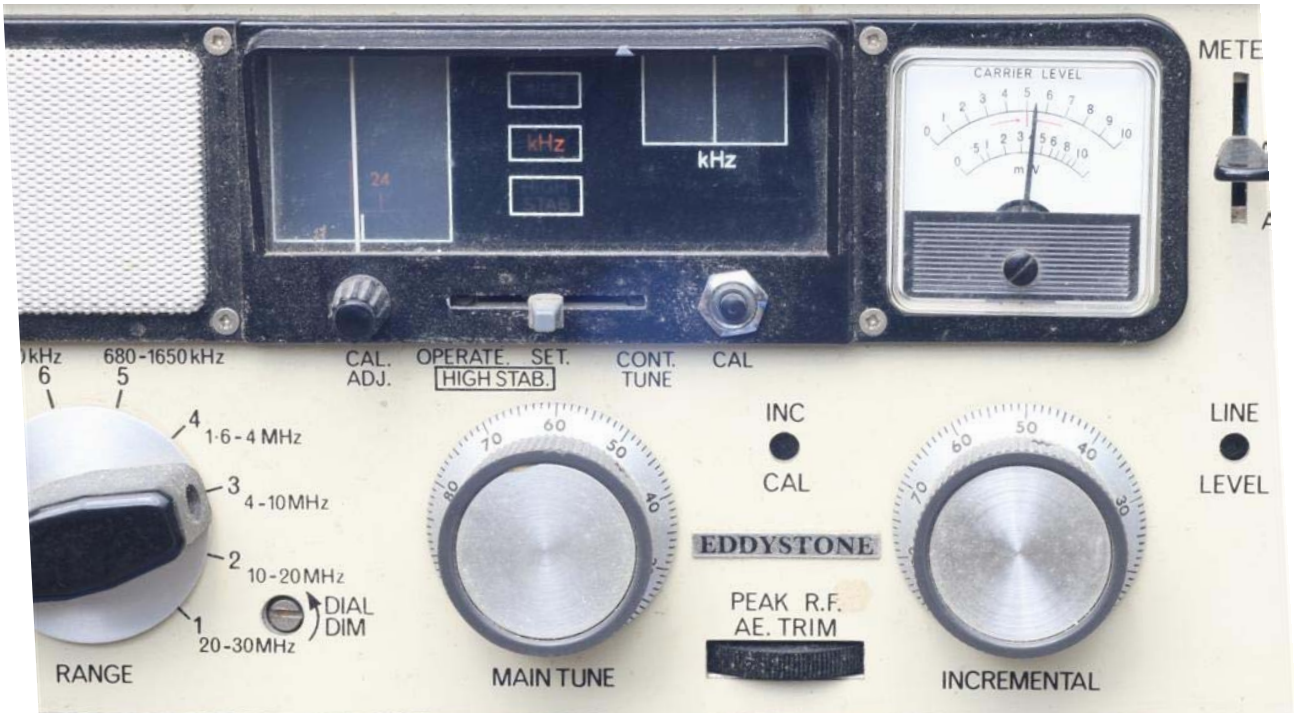
Above: close-up of the EC958 display panel. Below: Same view of the EC958/3 – note the 'cozy-looking' projection frequency display (very, er... 'valvey')
