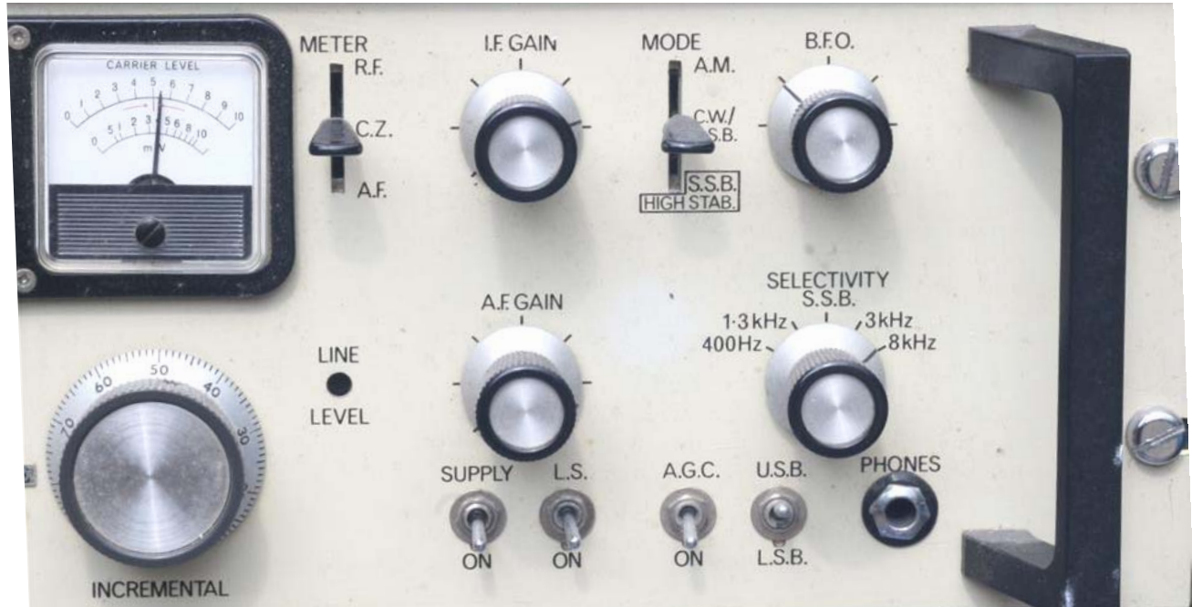
Above: close-up of the EC958 gain controls, Meter switch, Mode switch, Selectivity, BFO, and switch bank. Below: some more Wadley Loop 'trannies' mentioned in this article – clockwise from top left are the Yaesu FRG7, Standard C6500, Drake SSR-1 and Realistic DX-300
