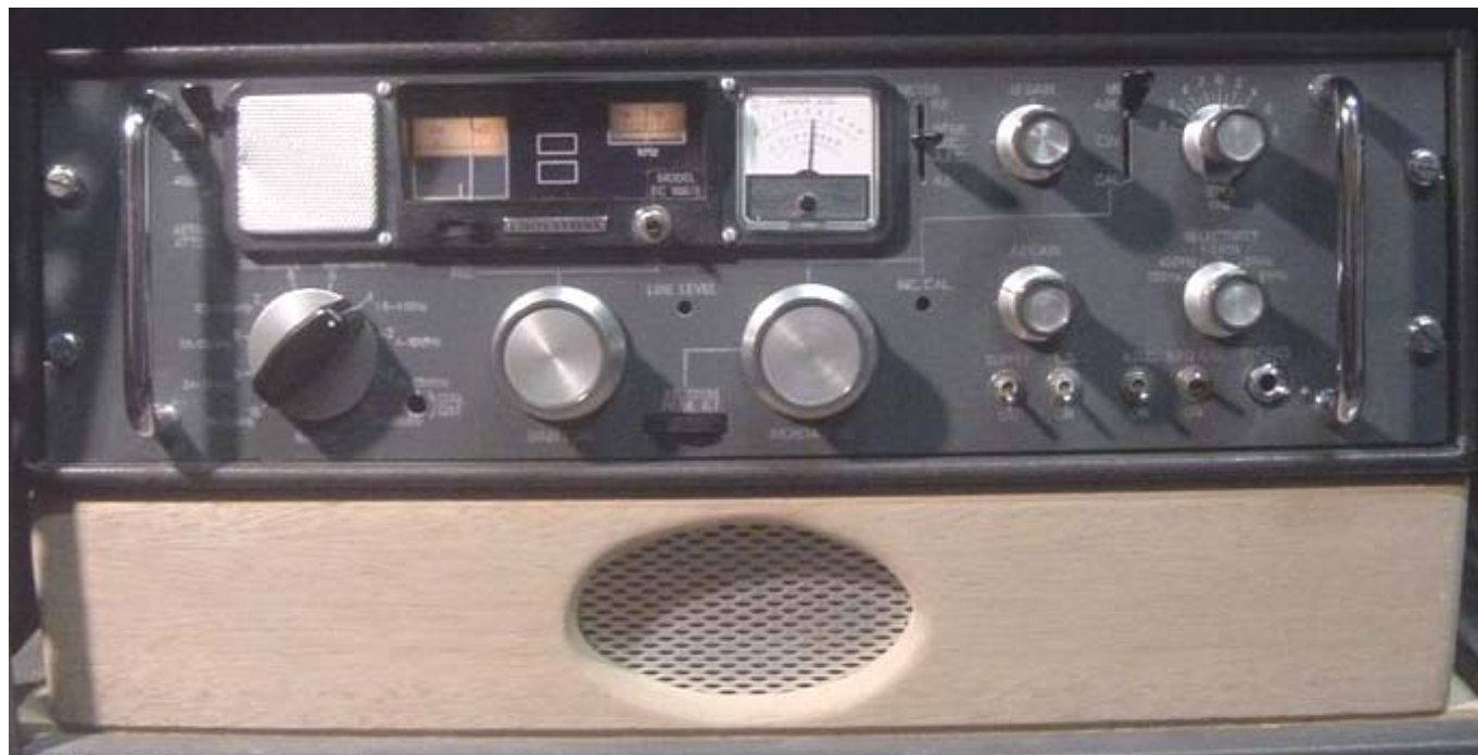
Above: front panel of the EC958/3 – the set sitting proudly on the well-built homebrew wooden plinth speaker it was supplied with (I must get around to spraying it black...) Below: a slightly later model EC958 – not just a colour scheme and handles change here – look carefully at the legends on the Mode and Selectivity switches. Also, note the absence of the 'Operate-Hi Stab-Cont Tune' switch on the display bezel on the EC958/3 above (see next page for close-up)
